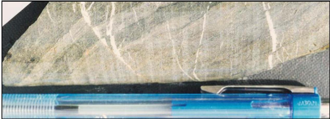
Figure 12 Phyllonite (PUS) with typical anastomosing S1 fabric transected and offset by late brittle veins with white carbonate infill (LED002 109.7m).
